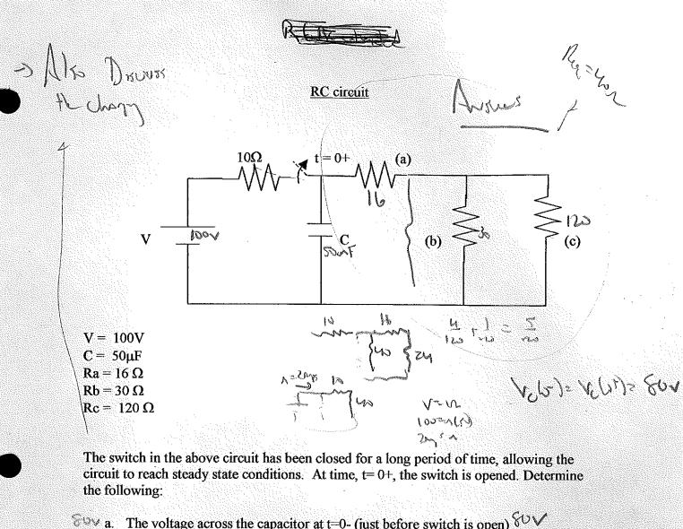
The voltage across the capacitor at t=0- (just before switch is open) b. The current down the capacitor branch at t=0- (just before the switch is open) C
