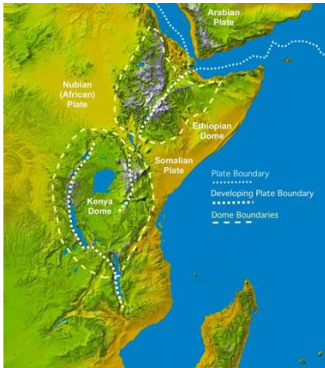
Figure 1: Colored Digital Elevation Model showing tectonic plate boundaries, outlines of the elevation highs demonstrating the thermal bulges and large lakes of East Africa.
