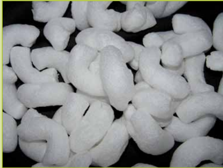
This foam packaging is made from cornstarch. It will dissolve in water.
